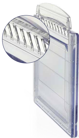
Figure 5. Unique wedge-shaped well design of Bolt Bis-Tris Plus gels. The WedgeWell feature enables larger sample loads and easier loading.
